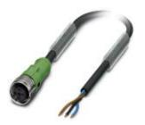
Sensor/Actuator cable, 3-position, PUR halogen-free, black-gray RAL 7021, free cable end, on Socket straight M12 SPEEDCON, A-coded, Cable length: 3 m
