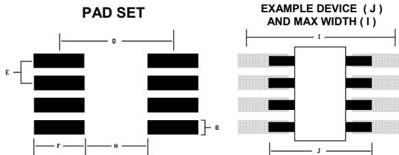
MOUNTING PADS ARE OVERSIZED IN LENGTH TO ACCEPT A WIDER RANGE OF DEVICE WIDTHS AND TOLERANCES AND TO PERMIT HAND SOLDERING.
