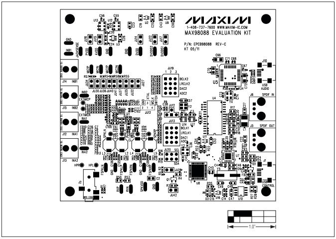
Figure 5. MAX98088 EV Kit Component Placement Guide—Component Side
