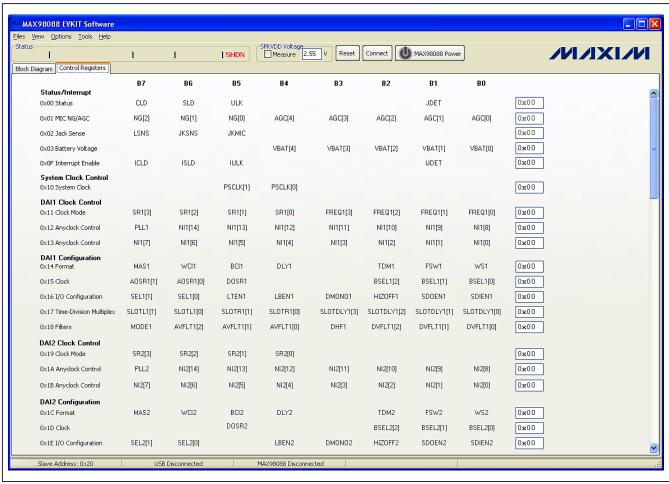
Figure 3. MAX98088 EV Kit Software Main Window (Control Registers Tab)
