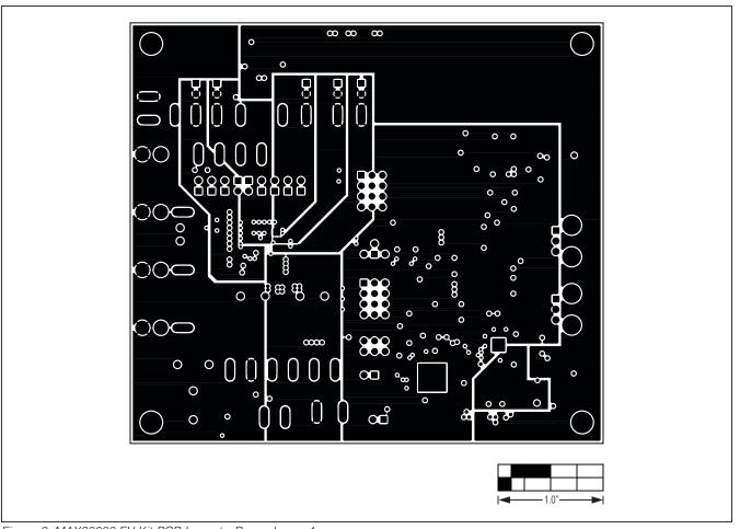
Figure 9. MAX98088 EV Kit PCB Layout—Power Layer 4
