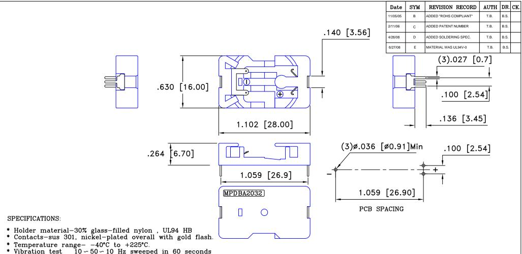
X,Y,Z direction 1 hour each direction Result: No dislodgement of the cell or damage No discontinuity over 10 micro-seconds.
