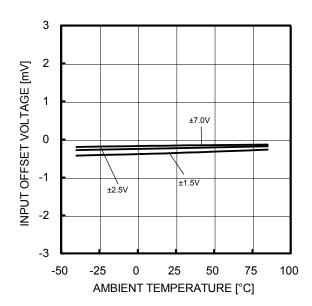
$\begin{array}{c} Figure \ 34. \\ Input \ Offset \ Voltage \ - \ Ambient \ Temperature \\ (V_{ICM} = 0V, \ VOUT = 0V) \end{array}$
