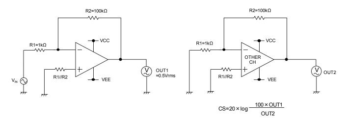
Figure 51. Test circuit 3(Channel Separation) (VCC=+2.5V, VEE=-2.5V)
