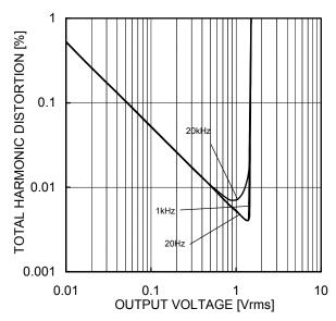
Figure 45. Total Harmonic Distortion - Output Voltage (VCC/VEE=2.5V/-2.5V,  $R_L$ =3k $\Omega$  80kHz-LPF,  $T_A$ =25°C)
