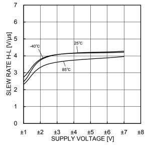
Figure 21. Slew Rate H-L - Supply Voltage
