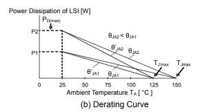
Figure 52. Thermal Resistance and Derating Curve
