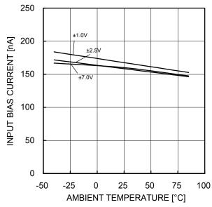
Figure 13. Input Bias Current - Ambient Temperature  $(V_{\text{ICM}}=0V,\ VOUT=0V)$
