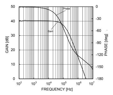
$\label{eq:figure 24.} Figure 24. \\ Voltage Gain - Frequency \\ (VCC/VEE=2.5V/-2.5V, Av=40dB, R_L=10k\Omega)$
