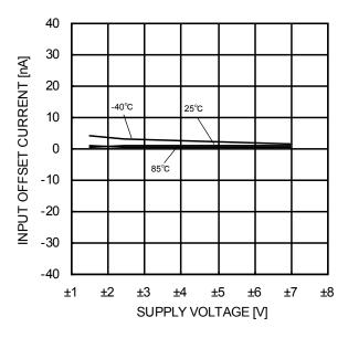
Figure 37. Input Offset Current - Supply Voltage  $(V_{ICM}=0V, VOUT=0V)$
