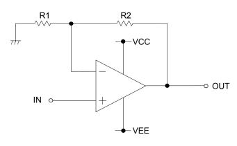
Figure 56. Non-inverting Amplifier Circuit
