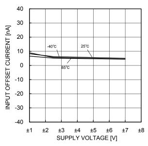
Figure 14. Input Offset Current - Supply Voltage  $(V_{\text{ICM}}=0V, VOUT=0V)$
