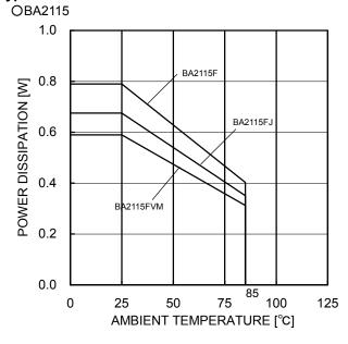
Figure 25. Derating Curve
