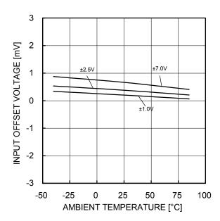
Figure 11. Input Offset Voltage - Ambient Temperature  $(V_{\text{ICM}}=0V, VOUT=0V)$
