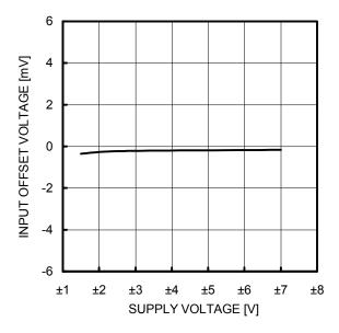
Figure 33. Input Offset Voltage - Supply Voltage  $(V_{ICM}=0V, VOUT=0V)$
