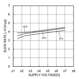
Figure 43. Slew Rate L-H - Supply Voltage
