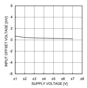
Figure 10. Input Offset Voltage - Supply Voltage  $(V_{\text{ICM}}=0V, VOUT=0V)$
