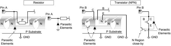
Figure 57. Example of monolithic IC structure
