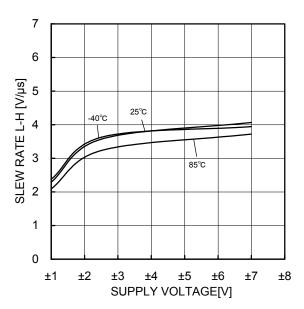
Figure 20. Slew Rate L-H - Supply Voltage
