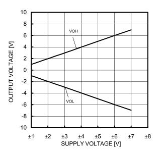
Figure 29. Maximum Output Voltage - Supply Voltage  $(R_L=10k\Omega)$
