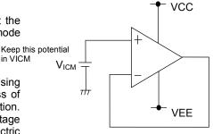
Figure 58. Example of Application Circuit for Unused Op-amp
