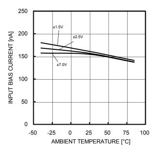
Figure 36. Input Bias Current - Ambient Temperature  $(V_{ICM}=0V,\ VOUT=0V)$
