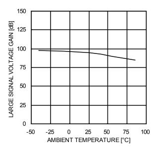
Figure 40. Large Signal Voltage Gain - Ambient Temperature (VCC/VEE=+2.5V/-2.5V)
