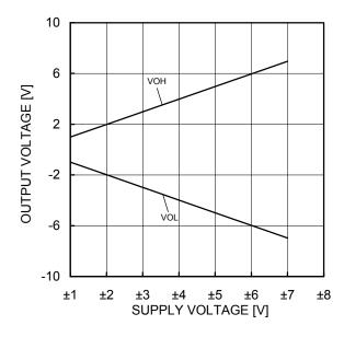
Figure 6. Output Voltage - Supply Voltage  $(R_L=10k\Omega)$
