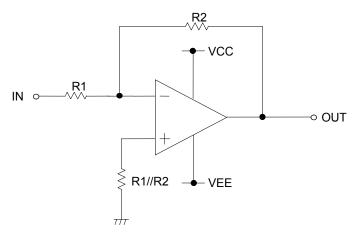
Figure 55. Inverting Amplifier Circuit
