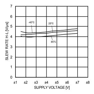
Figure 44. Slew Rate H-L - Supply Voltage
