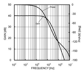
Figure 47. Voltage Gain - Frequency (VCC/VEE=2.5V/-2.5V, Av=40dB,  $R_L$ =10k $\Omega$ )
