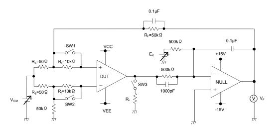
Figure 48. Test circuit1 (one channel only)
