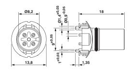
M12 female connector contact carrier
