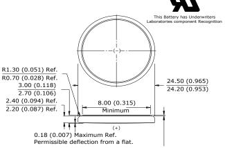
0.10 (0.004) Minimum Ref. (Applies to top edge of gasket or edge of crimp, whichever is higher.)
