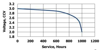
Classification: "Lithium Coin" **Chemical System:** Lithium / Manganese Dioxide (Li/MnO<sub>2</sub>) **Designation:** ANSI / NEDA-5011LC, IEC-CR2425 **Nominal Voltage:** 3.0 Volts
