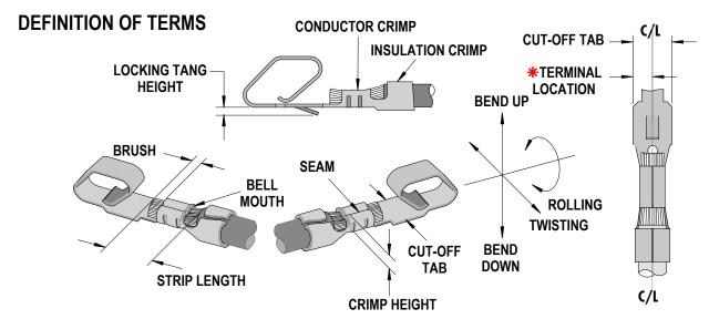
\* Terminal is to be centrally located between the two (2) cut-off tab edges by one half of the total cut-off tab tolerance.
