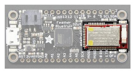
Since not all pins can be brought out to breakouts, due to the small size of the Feather, we use these to control the BLE module
