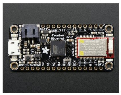
At the Feather 32u4's heart is at ATmega32u4 clocked at 8 MHz and at 3.3V logic, a chip setup we've had tons of experience with ais the same as the Flora (http://adafru.it/dVI). This chip has 32K of flash and 2K of RAM, with built in USB so not only does it have a USB-to-Serial program & debug capability built in with no need for an FTDI-like chip, it can also act like a mouse, keyboard, USB MIDI device, etc.
