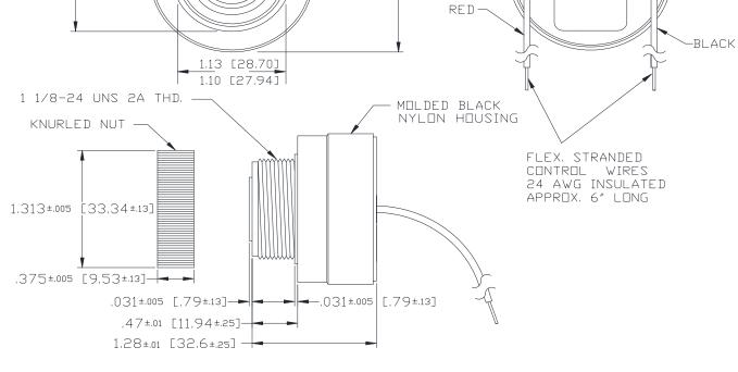
NOTE: MOUNTING- REMOVE BLACK PLASTIC NUT AND INSERT THREADED FRONT THROUGH 1.25" HOLE PUNCHED IN PANEL, IF ORIENTATION IS NEEDED, NOTE LOCKING FLATS ON DRAWING. SCREW NUT BACK ON. DO NOT OVERTIGHTEN.
