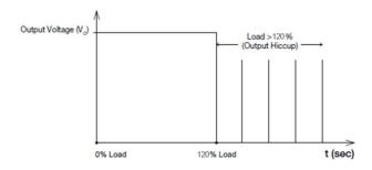
Additionally, if the  $I_0$  is < 120% but > 100% for a prolong period of time (depending on the load), the Over Temperature Protection (OTP) will be activated due to high temperature on critical components. The power supply will then go into "Hiccup mode" until power supply cool down.
