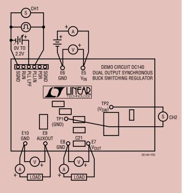
Figure 3. Proper Measurement Setup
