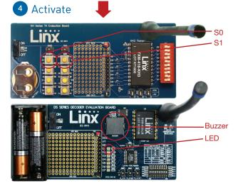
Push S0 to activate buzzer and push S1 to turn on the LED.
