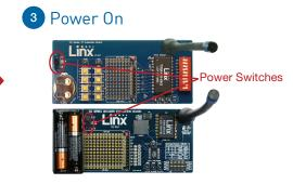
Turn on the power switch on each board.
