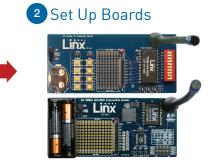
Install batteries and an antenna on each board.
