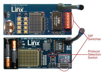
Ensure the DIP Switches are set the same. All switches on and all switches off are not valid settings. At least 1 must be different.
