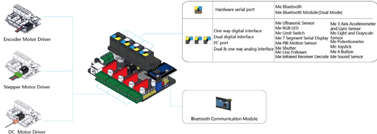
Wireless communication interface – for adding Bluetooth module or 2.4G module (require corresponding communication module)
