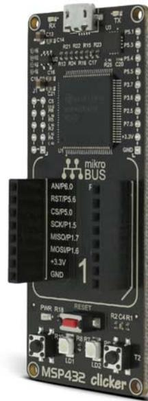
**MSP432 clicker** is a compact development board with a mikroBUS™ socket for click board connectivity. It carries the SimpleLink™ MSP432™ - ARM® 32-Bit Cortex®-M4F CPU with integrated 1Msps 14-bit SAR-based ADC from **Texas Instruments**.
