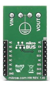
**Boost 4 click** carries the TPS61230A, a high efficiency fully integrated synchronous boost converter from Texas Instruments. The click is designed to run on a 3.3V power supply. Boost 4 click drives the target chip through the digi pot, which has SPI communication with the microcontroller on the system.
