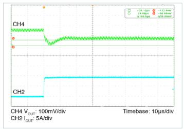
Figure 13 — Load transient response, nominal line Load step 0–25%
