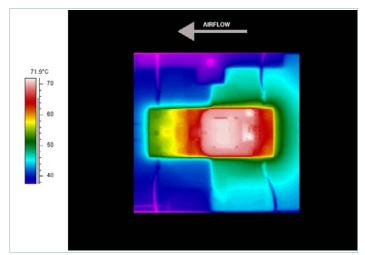
**Figure 26** — Thermal plot, 200LFM, 25°C, 48V<sub>IN</sub>, 300W output power
