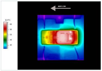
**Figure 28** — Thermal plot, 400LFM, 25°C, 48V<sub>IN</sub>, 300W output power
