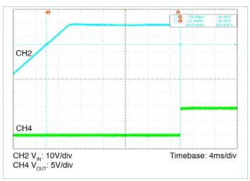
**Figure 7** — Turn on delay time; V<sub>IN</sub> turn on delay at nominal line, 15% load; Start-up inhibit time
