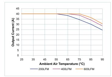
**Figure 19** — Output current derating vs. ambient air temperature at V<sub>IN</sub> nominal. Transverse airflow. Board and junction temperatures within IPC-9592 derating guidelines
