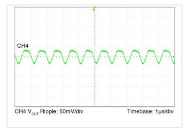
Figure 16 — Output ripple; nominal line, full load
