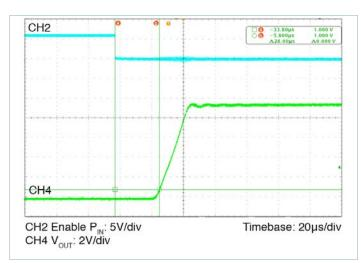
**Figure 8** — Turn on delay time; Enable turn on delay at nominal line, 15% load. Also illustrates V<sub>O</sub> overshoot at turn-on.
