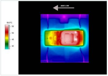
**Figure 30** — Thermal plot, 600LFM, 25°C, 48V<sub>IN</sub>, 300W output power
