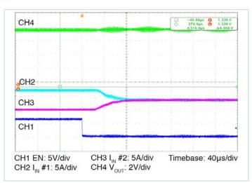
**Figure 18** — Two modules parallel array test.  $V_{OUT}$  and  $I_{IN}$  change when one module is enabled. Nominal  $V_{IN}$ ,  $I_{OUT} = 40A$
