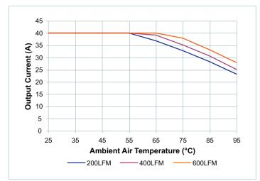
**Figure 20** — Output current derating vs. ambient air temperature at V<sub>IN</sub> nominal. Longitudinal airflow. Board and junction temperatures within IPC-9592 derating guidelines
