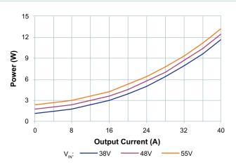
Figure 4 — Power dissipation vs output current, 25°C ambient
