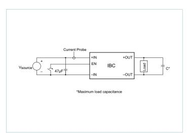
Figure 22 — Test circuit; inrush current overshoot
