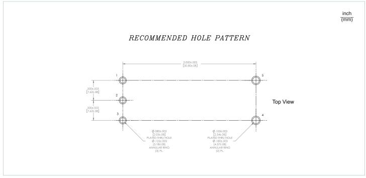
Figure 33 — IBC PCB recommended hole pattern
