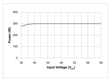
Figure 21 — Maximum output power vs. input voltage
