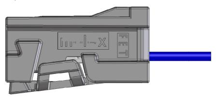
Do not force the ISL closed! damage to the terminal and connector ISL will occur
