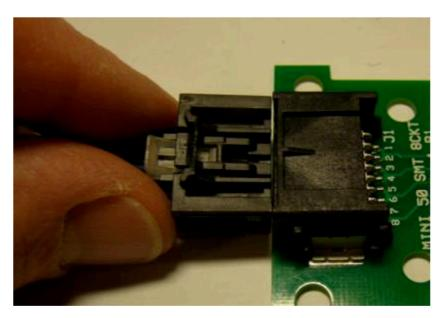
After mating the connector, push on the CPA to engage
