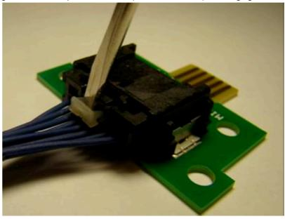
Push the connector together to unload the latch system. Depress the latch and hold. Gently pull the connectors assemblies apart
