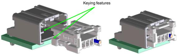
If resistance is encountered, confirm the ISL is fully locked and all terminals are fully installed. A partially installed terminal will not allow the ISL to close.
