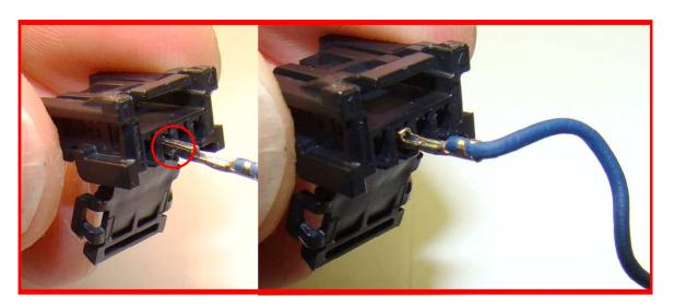
Terminal improperly inserted 180° NOTE WIRE BUCKLE
