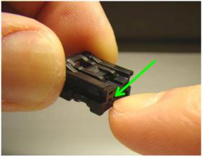
To verify the ISL is fully latched gently pull down here after closing
