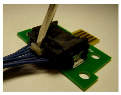
Push the connector together to unload the latch system. Insert a small flat tip screwdriver (width 2-2.5mm) between the latch and the latch cover.
