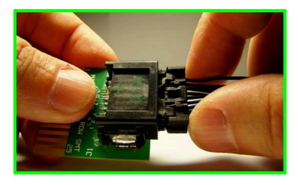
Always push on connector housing while mating. DO NOT push on latch while mating.
