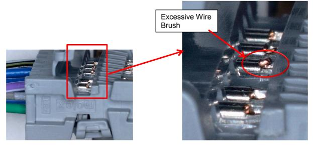
**BAD** - ISL Bowing caused by excessive wire brush:
