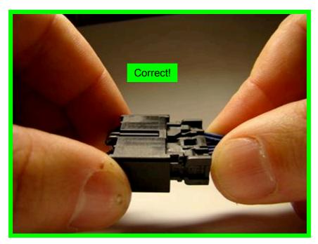
Never mate system at an angle, or with bias. This may cause damage to the header, or connector.
