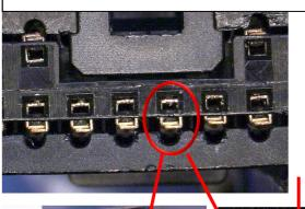
GOOD: Terminals correctly crimped and positioned – No ISL Bow
