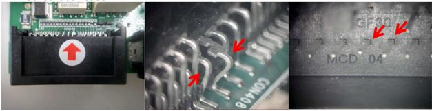
A2. ISL Bow (due to improperly crimped and/or bent terminals):
