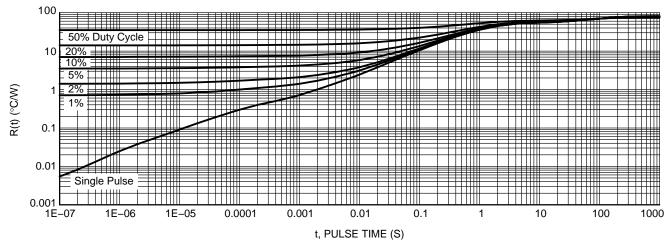
Figure 8. Typical Transient Thermal Response Characteristics, Junction-to-Ambient
