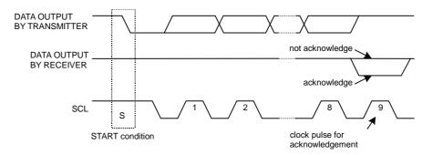
Figure 8. Acknowledge (I<sup>2</sup>C format)
