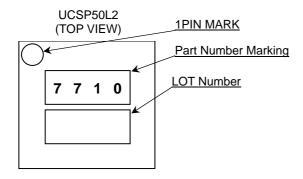
Figure 35. Marking Diagram
