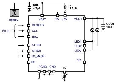
Figure 1. 1.5A application Block diagram
