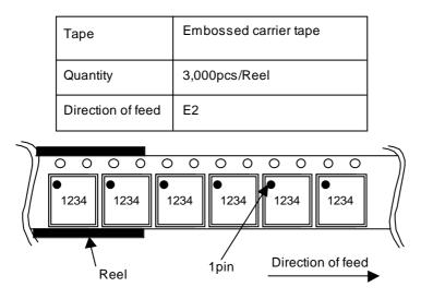
Figure 34. Typical Tape and Reel configuration
