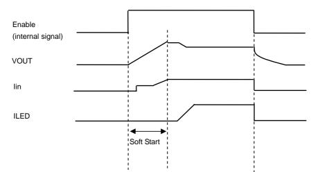
Figure 15. Soft Start with enable signal
