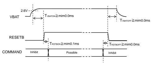
Figure 13. Power up/down sequence
