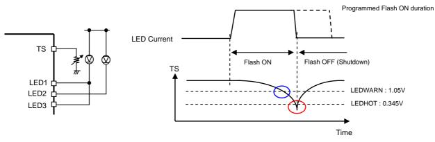
Figure 26. Sensing the LED Temperature
