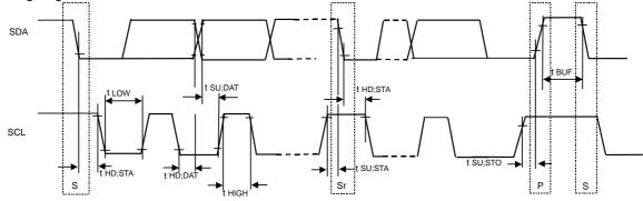
Figure 12. Timing diagram (I<sup>2</sup>C format)
