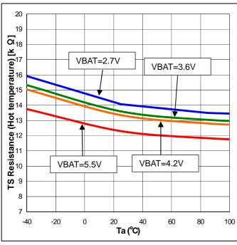
Figure 5-13. TS Resistance (Hot temperature) – Temperature
