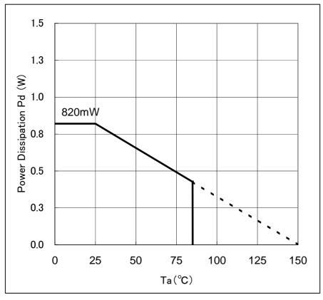
Figure 33. Power dissipation
