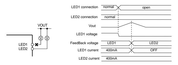
Figure 24. LED open Protection
