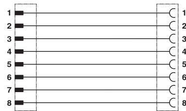
Contact assignment of M12 connector/socket
